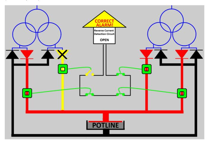
The LKAT will detect the reverse current in the yellow bus bar (reverse current coming from the other parallel rectifiers) and 'open' its dry contact. Because all Reverse Current Detection Circuit contacts are wired in series, the overall circuit will 'open' signaling a reverse current event. This is used to trip all rectifiers off line to minimize damage.
