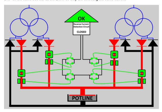
The LKAT ( ) and BRP ( ) do not interfere with or influence each other in any way so they can be installed immediately next to each other. Like the LKAT, the BRP controls its own relay / dry contact that is wired in 'parallel' with the original LKAT relay / dry contact.
