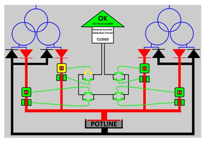
However, as illustrated above, a false alarm from one system ( LKAT in the example above ) will <u>not</u> cause a false alarm. The power rectifiers will not be tripped off line so the process can continue without interruption.
