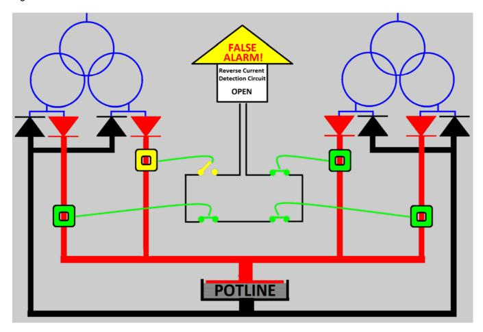
Extreme bus bar electrical noise, component failure, significant mains power noise or loss of power to an LKAT could cause a false trip depending on how it is configured. This is noted by the yellow LKAT in the diagram above. This false detection opens the overall circuit signaling a reverse current event which trips all rectifiers off line.
