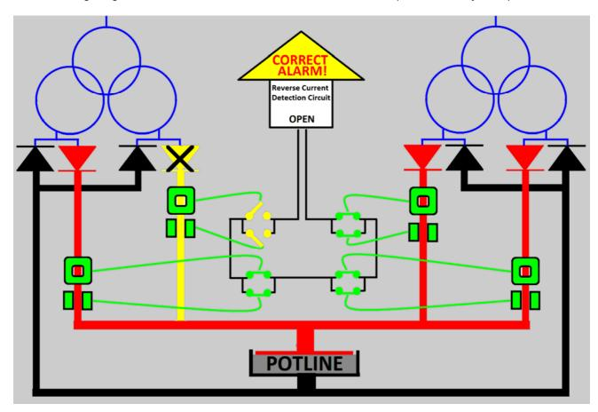
BOTH the LKAT and the BRP will detect the reverse current in the yellow bus bar (reverse current coming from the other parallel rectifiers). Each will 'open' its dry contact accordingly. With both contacts open, the overall Reverse Current Detection Circuit will 'open' to trip all rectifiers off line to minimize damage.
